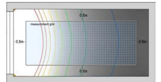
Figure 4 Daylight factor calculation
